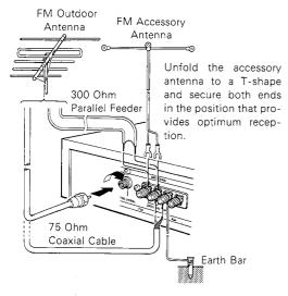
**CAUTION**: Never make a connection to a gas pipe because it can cause a fire hazard.
